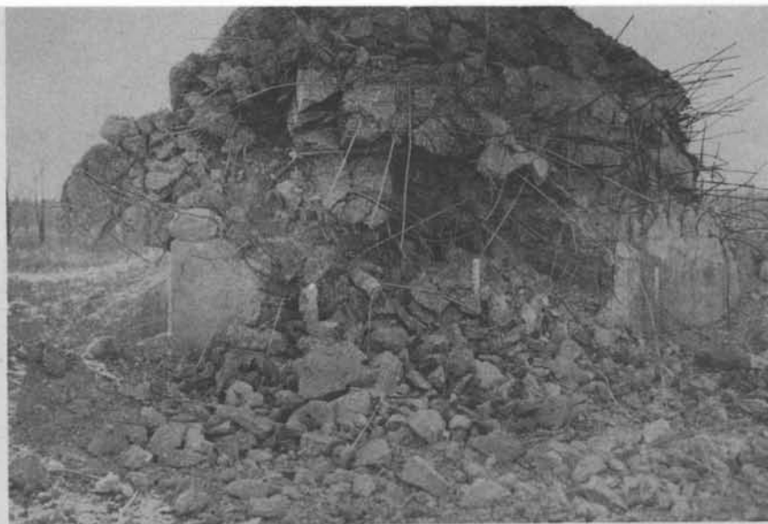
Gun, 155 mm, M1A1, firing Shell, H.E., 155 mm, M101, with Fuze, CP, M78. Range using normal charge point blank range. View of damage to German-type reinforced concrete pillbox resulting from two rounds of shell.
